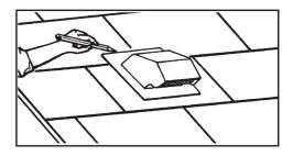
Step 2: Trace the outline of the flange onto the shingles. Cut a hole through the roof decking slightly larger than the diameter of the duct.
