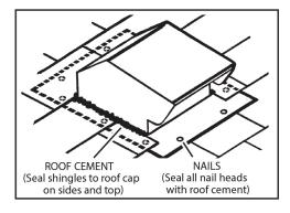
Step 4: Carefully lift the shingles while sliding back the flange under the lifted shingles. Nail the flange to the roof on top and two sides. Nail the bottom on top of the shingles directly to the roof. Use roofing cement to seal the shingles to the top and two sides of the vent to prevent leakage. Seal the nail heads using roofing cement.
