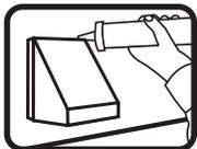
Secure to outside wall using 4 screws (not included). Caulk around the vent frame and wall if necessary.
