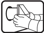
From the outside, slide the pipe (if applicable) through the hole opening until the vent is flush against the outside wall surface.
