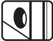
Cut a hole 1/2" larger than the pipe through the outside wall or use an existing hole.
